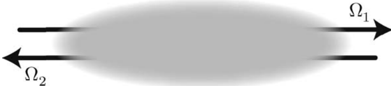
Figure 12.8 Two counterpropagating and overlapping laser beams interact with a cloud of cold atoms.
