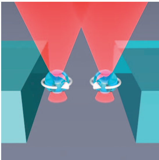
Figure 9.5 Applications of rotational control in optical tweezers. Leach and colleagues used counter-rotating vaterite spheres placed in a microfluidic channel to generate an optically driven micropump.
